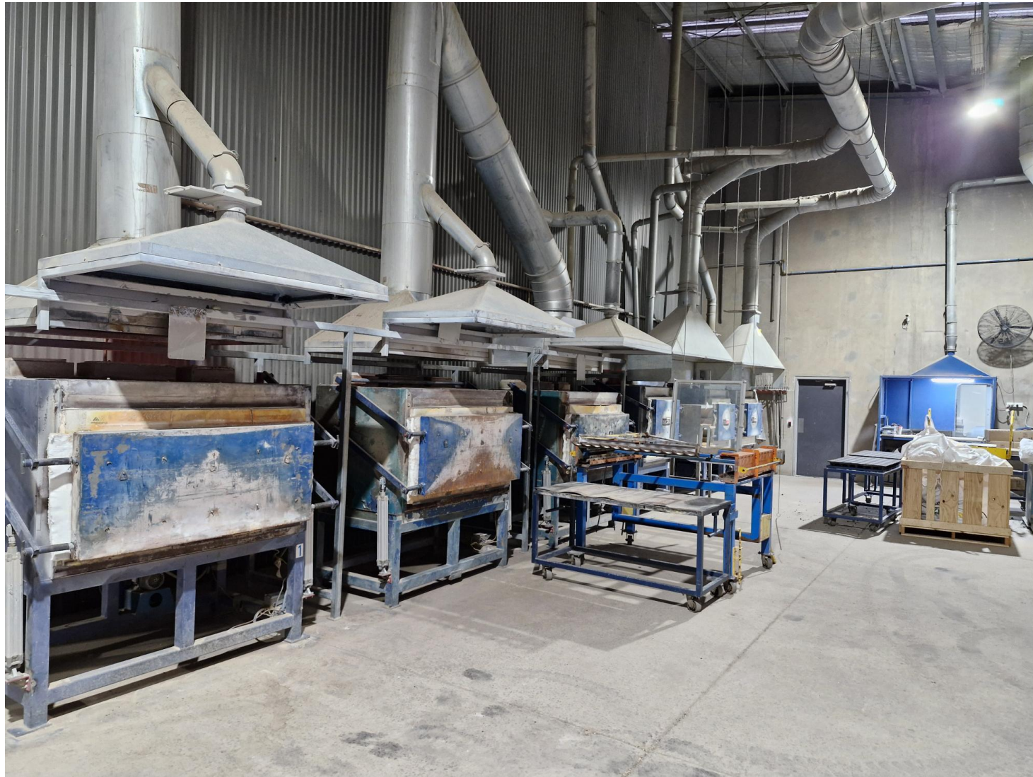
Figure 8 Three furnaces (left) heated to 1050°C and two furnaces (right) heated to 950°C
